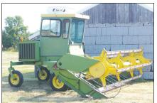
**JD Model 800 Swather.** 14' draper header, 6 cylinder gas motor
